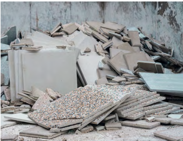
Demolition waste is collected, sorted and pulverised into aggregate chips for inclusion into new terrazzo products at our partner’s facility in Manchester.
