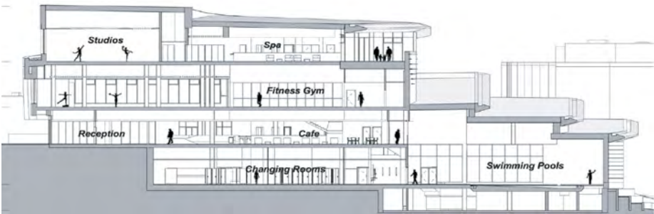
Section showing wet and dry areas
