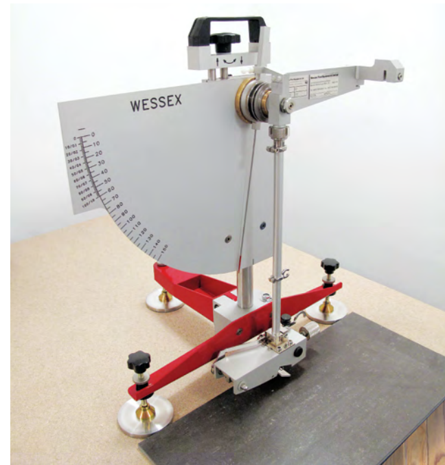
A Pendulum Test Value is measured with a piece of equipment called a pendulum machine. This equipment is used to simulate the action of a shoe or a bare foot by swinging different density rubber sliders across a section of flooring. Wet environments are simulated by spraying potable water onto the test surface, usually after a dry test has been performed.
