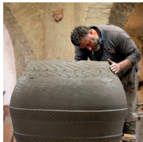
Handmade amphorae - some able to hold 600l – are still made using the "based-work" technique where the potter moves around the pot, rather than using a wheel. Galestro -rich clay comes from the quarry behind the factory.
