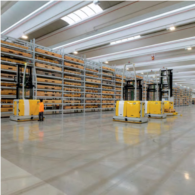
A fleet of 54 battery-powered, laser-guided vehicles transport maximum loads of 4 tonnes around the plant. With the installation of solar panelling, they will be recharged with renewable energy.
